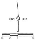
Tenn State Plane Coordinates (NAD 83), Elevations (NAVD88), and Tenn Grid Azimuth were determined using the City of Crossville's cell phone reference station at @ N588,647.937' E2,256,110.694' EL1,857.54'
